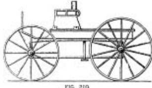
invention consists in an improved track arranged upon the top rail of the wagon body, and in the opposite holding plates for the seat.
